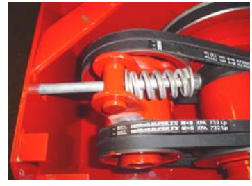
6) Bolt for thightener to be mounted with feder and thightened. To be tightened until feder has 45 mm left.
