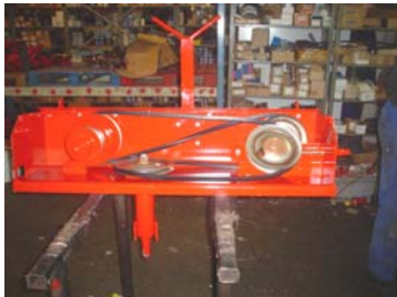
4) around tightening pulley and V-belt must be tightened.
